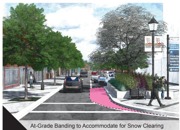
At-Grade Banding to Accommodate for Snow Clearing
