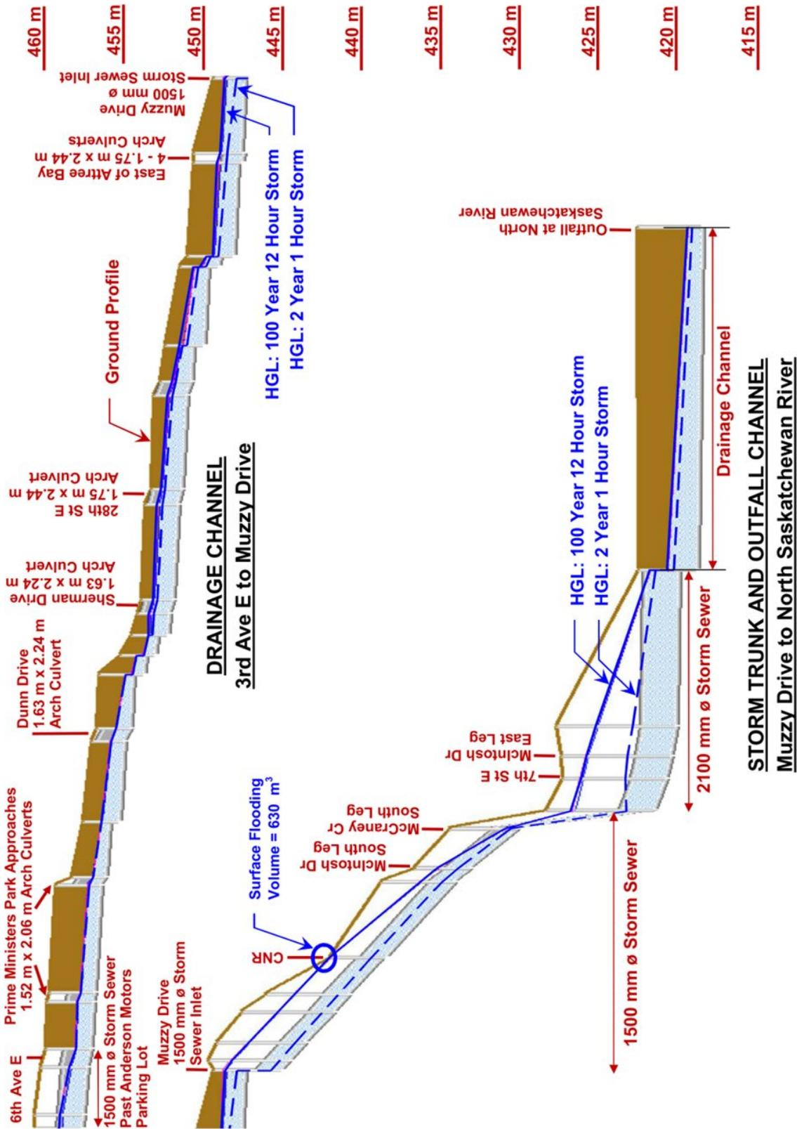
Figure 9.2: Drainage Ditch and Storm Trunk - 3rd Avenue East to Outfall at North Saskatchewan River
