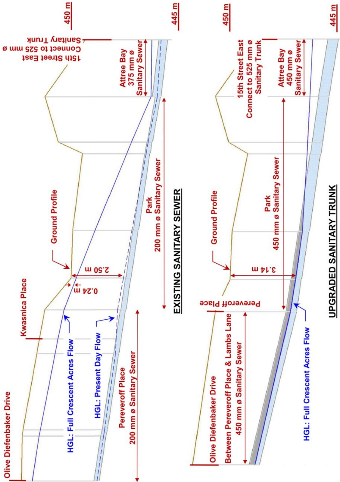
Figure 7.2: Sanitary Sewer from Olive Diefenbaker Drive to 15th Street East
