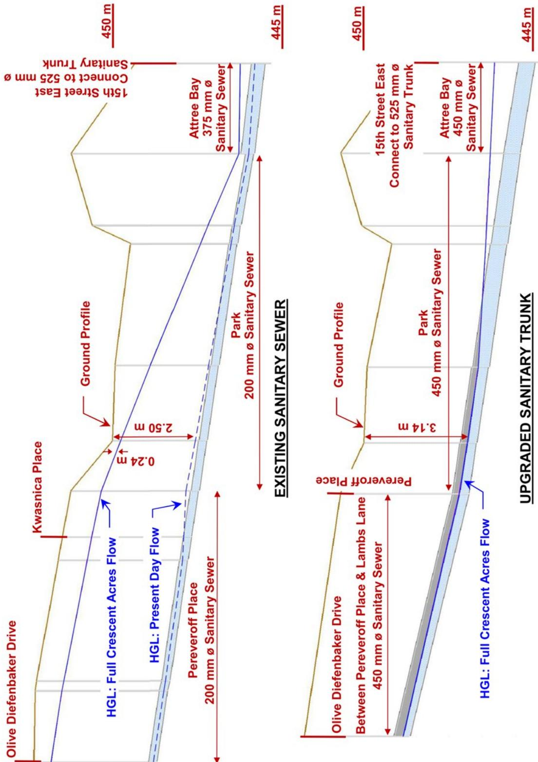
Figure 7.1: 15th Avenue East Sanitary Trunk (525 mm  $\varnothing$ ) from 28th Street East to 7th Street East
