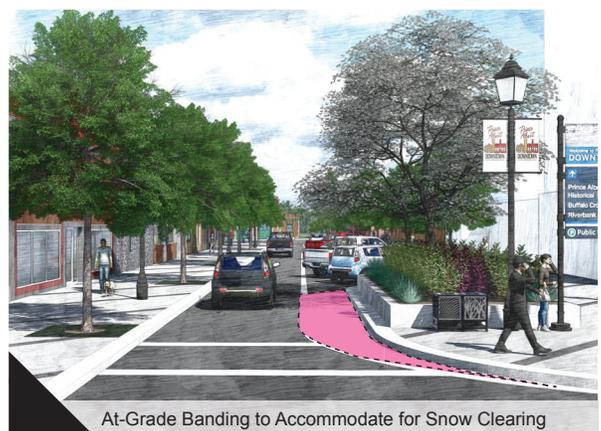
At-Grade Banding to Accommodate for Snow Clearing
