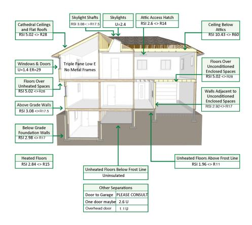
THE ABOVE AND BELOW GRADE FOUNDATION WALLS LISTED ABOVE ARE BASED ON 2X6 CONSTRUCTION SPACED 24" O.C. WITH A HRV (HEAT RECOVERY VENTILATION
