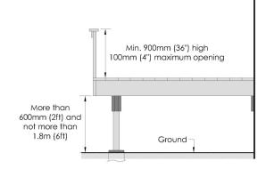
Figure 4: Guardrails for decks over 6 feet
